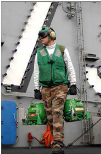
5 LITER LOX CONVERTER (REMOVABLE) NSN - 1660-00-327-7048 P/N - 10C-0020-9 PLATFORMS - F-16, F-15, F-5, F-4
