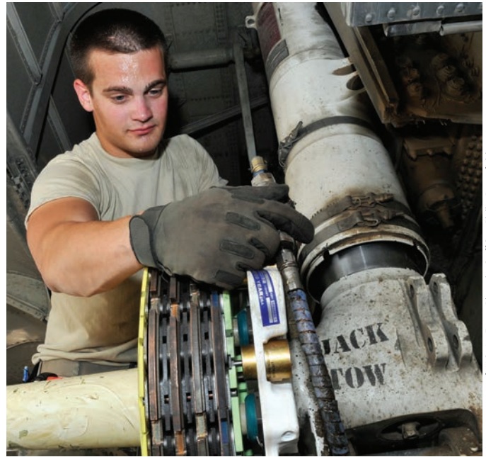
▲ Airman 1st Class Joel Rivera measures the height off the ground of C-130J Super Hercules landing gear during an isochronal inspection at Ramstein Air Base, Germany.
