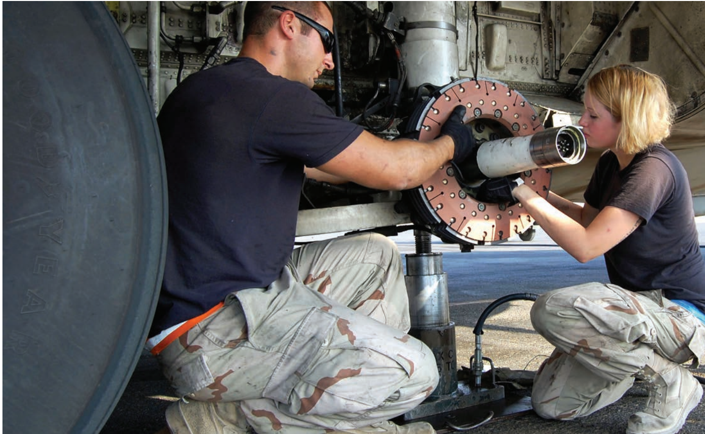
▲ Senior Airman Michael Bruke and Airman 1st Class Britney Warner install a multi-disc brake on a C-130E Hercules in Southwest Asia.
