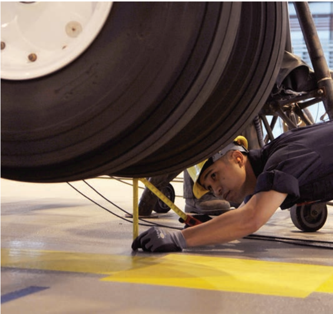
▲ Airman 1st Class Joel Rivera measures the height off the ground of C-130J Super Hercules landing gear during an isochronal inspection at Ramstein Air Base, Germany.
